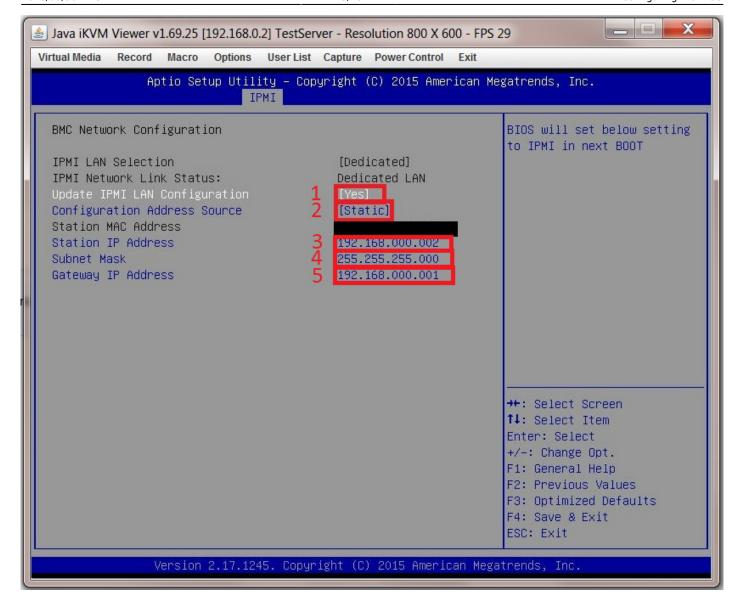
You have now assigned a static IP address to the IPMI web GUI. We will now always know where to find the IPMI GUI and it will not change even when the router gets rebooted.
