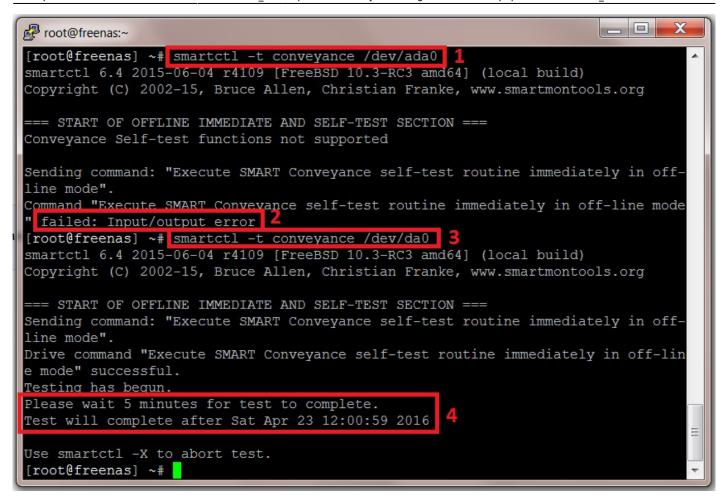
We now need to repeat this process for each drive in the system. We do not need to wait for this drive to complete its test before starting another on a different drive.
