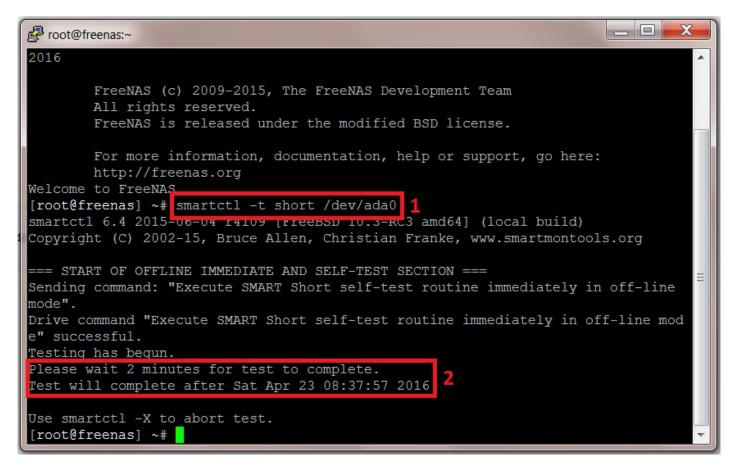
(Do not worry about the fact that you cannot see any results or the test running. This is completely correct. The results are obtained later by entering another command at the command prompt after all the tests are completed.)
