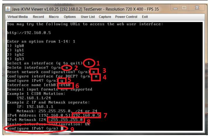
That's the static IP addresses assigned.
