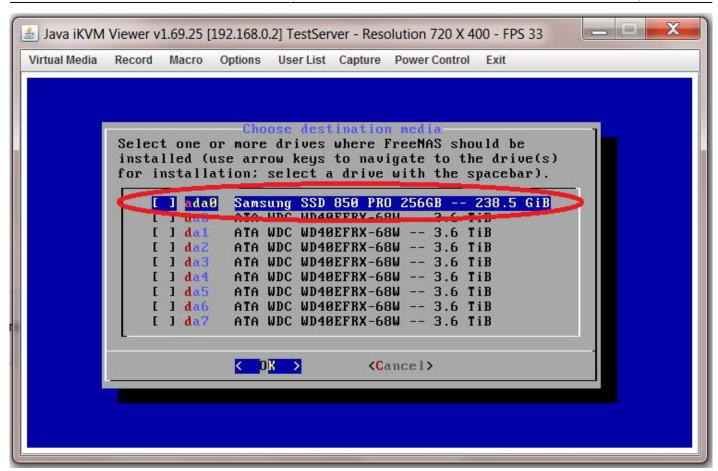
With the drive of your choice selected press the "Space Bar" key and an asterisk should appear next to the selected drive (1) now select "OK" (2) and press the "Return/Enter" key. If you want to install to two mirrored USB sticks, select them both and the installer will create the mirror.
