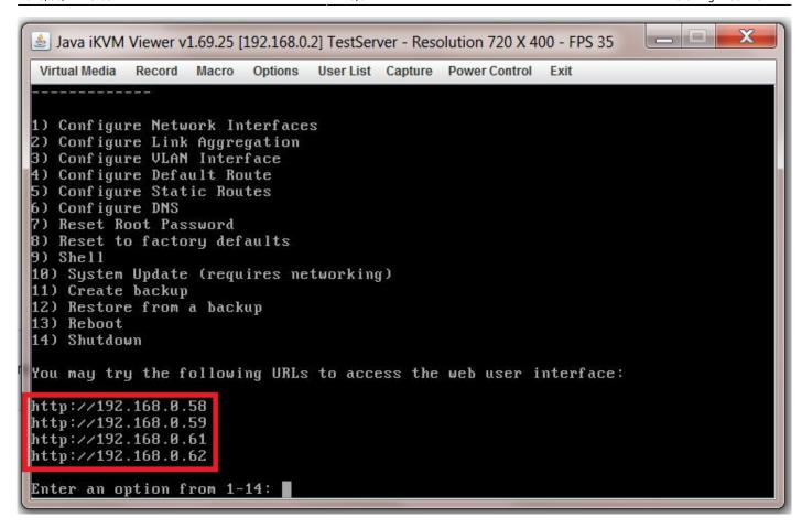
Make a note of the IP address/s for the FreeNAS web GUI, it will be needed soon.
